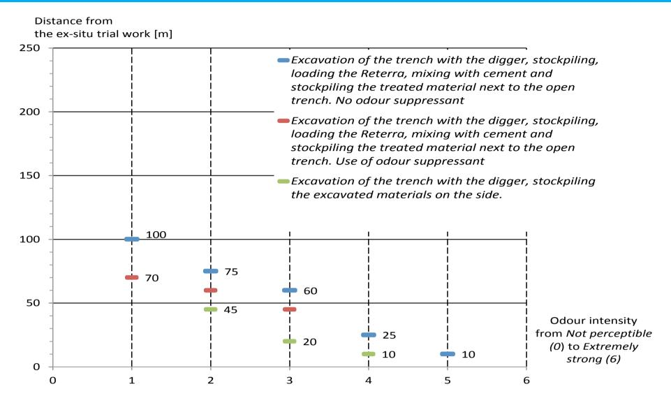
Weak odours were recorded over a narrower range of distances (between 70 and 100m) when compared with the in-situ trial. However the range of distances did not vary significantly when recorded odours were more intense.
